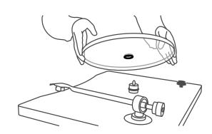
**Transmission belt:** switch the motor off. Fit the drive belt around the platter and the smaller diameter part of the motor pulley (33 1/3 rpm) or the bigger diameter of it (45 rpm).
